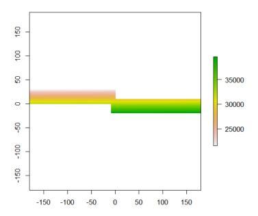
flip lets you flip the data (reverse order) in horizontal or vertical direction—typically to correct for a 'communication problem' between different R packages or a misinterpreted file. **rotate** lets you rotate longitude/latitude rasters that have longitudes from 0 to 360 degrees (often used by climatologists) to the standard -180 to 180 degrees system. With t you can rotate a Raster\* object 90 degrees.
